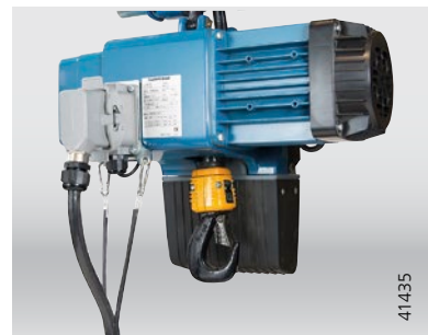
External connector for the control cable
