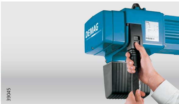
Height adjustment of the control cable
