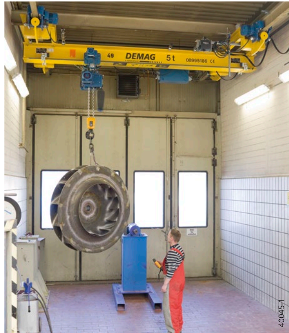
Minimum travelling chain hoist approach dimensions thanks to suspension crane end carriage based on DC chain hoist trolleys
