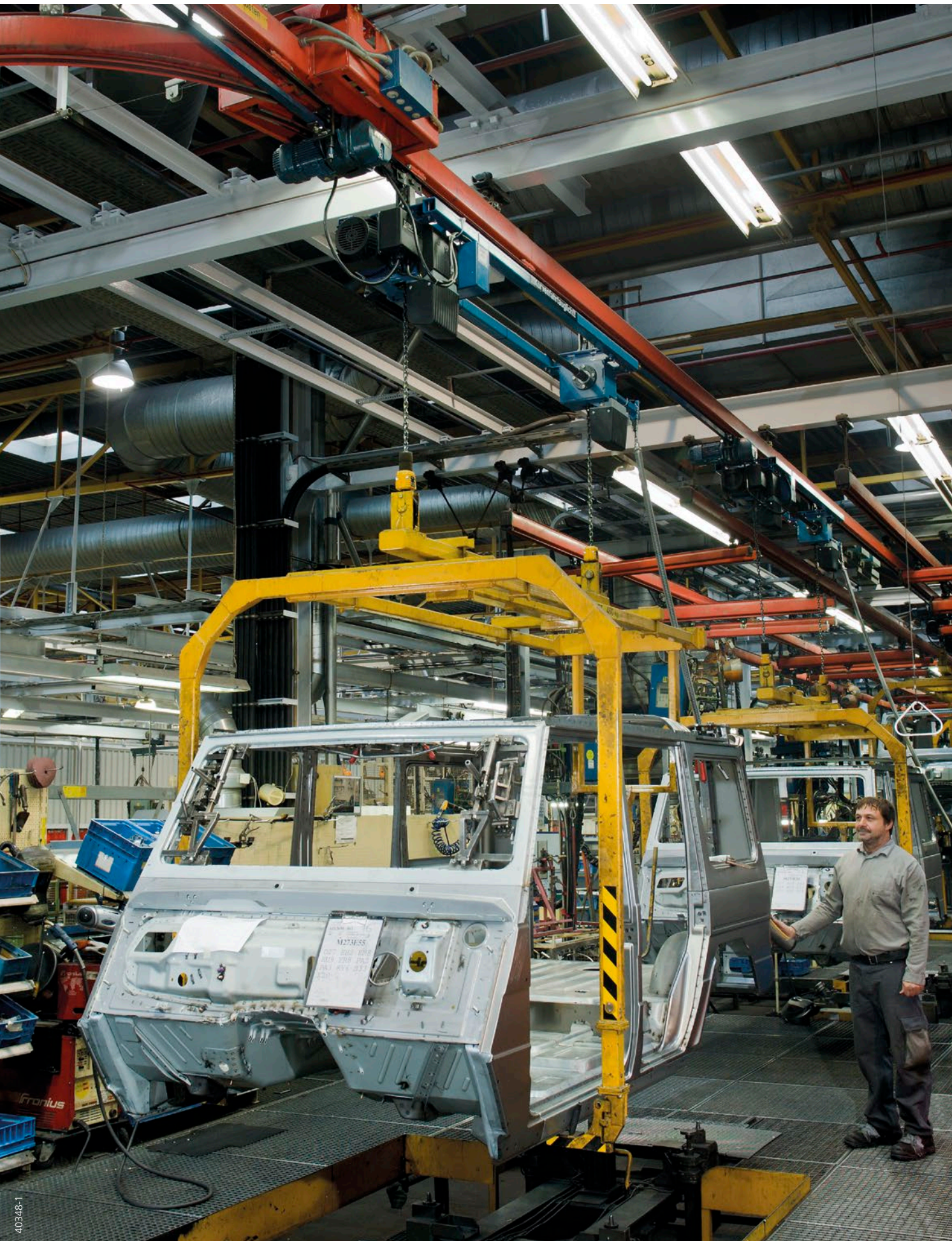
Car bodies being transported by two mechanically synchronised chain lead-offs on an LDC-D
