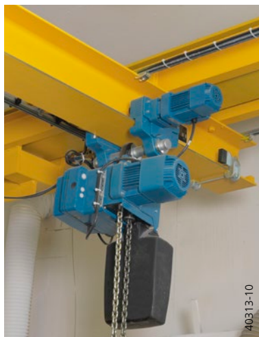
Operation on KBK with RF 125 friction wheel travel drive and E22-C travel drive
