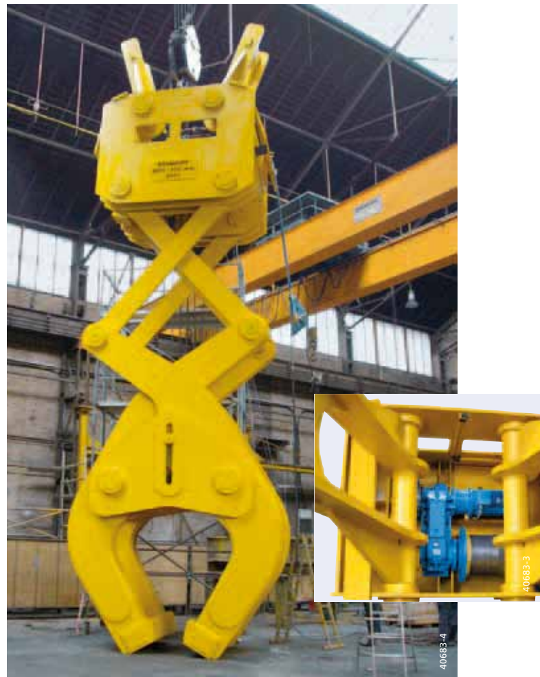
MPW open winch unit employed in a gripper system for transporting steel slabs
