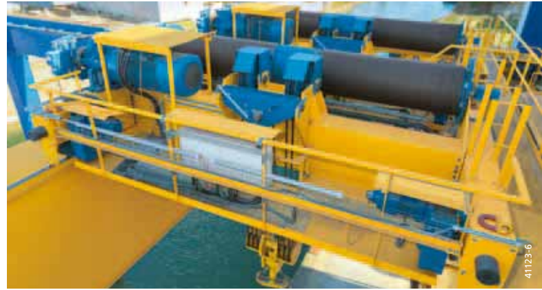
Two 125-tonne MPW crabs for quayside handling with weather-protection equipment for operation outdoors
